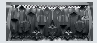
V ROTOR ► V rotor with two rows of blades.
