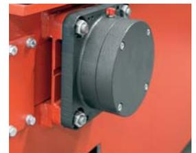
**OFFSET K BEARINGS** ▶ The offset K bearings are extremely low-wear and prevent the generation of heat.
