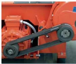
**DRIVE VIA ELECTRIC MOTOR** ▶ Drive up to 22 kW via V-belt and gearbox.
