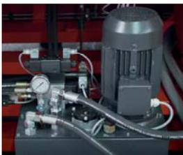
**HYDRAULICS IN THE MACHINE BODY** ▶ Is thus protected from synthetic dust and damage.
