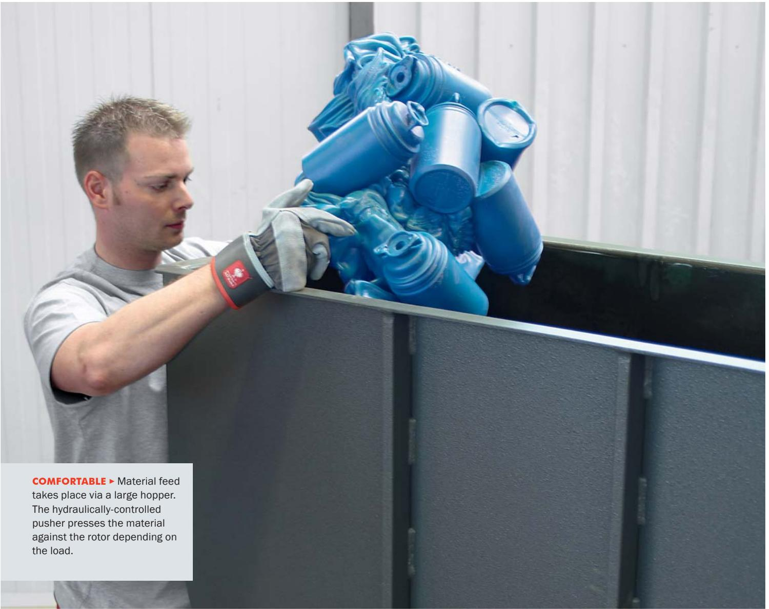
**COMFORTABLE** ▶ Material feed takes place via a large hopper. The hydraulically-controlled pusher presses the material against the rotor depending on the load.
